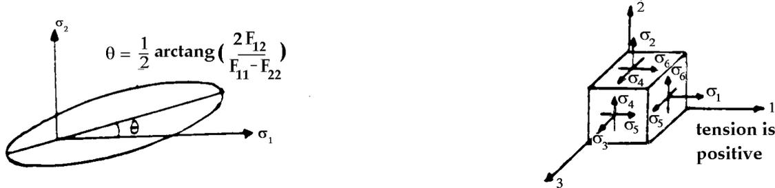
Figure 2.1. Failure ellipsoid and definition of positive stresses.
